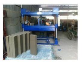
Mobile mold trays with bricks after cut96 bricks 7.5x 20 x60cm are cut nicely Note: some images may defer from the real machine. The Seller reserves the right to change the specifications without notice.
